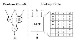
Figure 2: A function with  $\delta = 3$  input and  $\sigma = 1$  output bits represented as Boolean circuit with 2-input gates (left) and lookup table (right).
