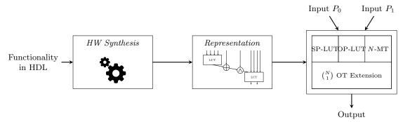
Figure 1: Our toolchain for compiling a high-level hardware description language into a network of 2-input Boolean gates and LUTs and evaluating them using our communication-efficient SP-LUT, OP-LUT, and N-MT protocols, which build on our improved  $\binom{N}{1}$  OT extension protocol.
