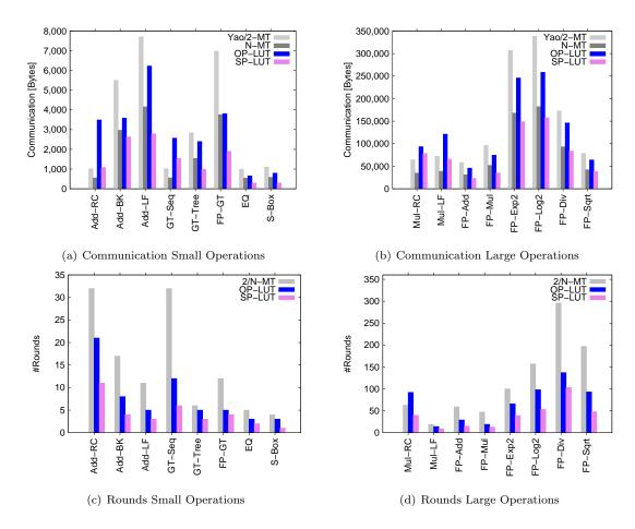
Figure 3: Total Communication (a,b) using Yao's garbled circuits (§2.4) and 2-MT (§2.5), our N-MT (§3), our OP-LUT ( $\delta \leq 4$  inputs, cf. §4.3) and our SP-LUT ( $\delta \leq 8$  inputs, cf. §4.4) and round complexity in the online phase (c,d) for a Boolean circuits evaluation using GMW (MT), OP-LUT, and SP-LUT for 32-bit operations and the 8-bit AES S-box. Yao's round complexity is constant and therefore not included.
