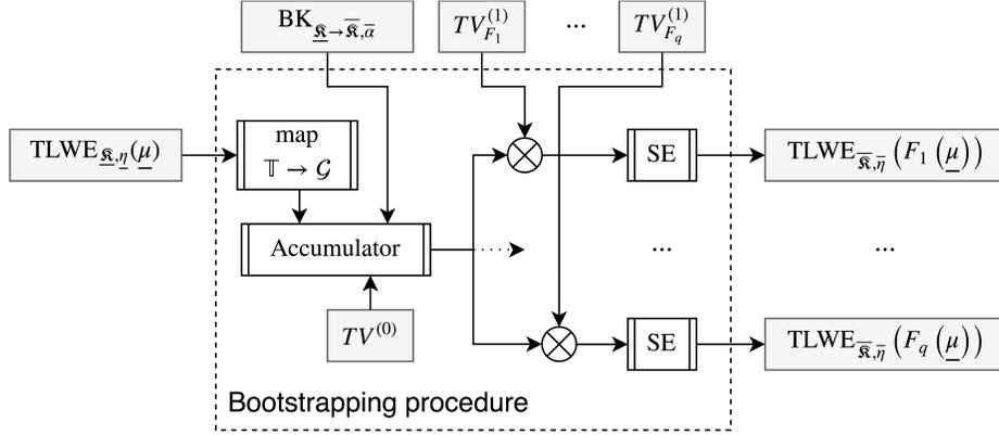
**Fig. 3.** Multiple output multi-value bootstrapping overview. Test polynomials  $\text{TV}_{F_1}^{(1)}, \dots, \text{TV}_{F_q}^{(1)}$  correspond to  $q$  functions evaluated over message  $\underline{\mu}$  encrypted in the input ciphertext.
