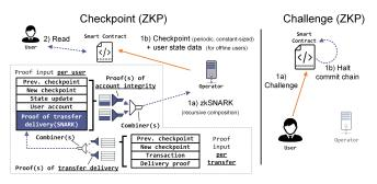
Fig. 4: High-level overview of the *Checkpoint* and *Challenge* sub-protocols in NOCUST-ZKP. The checkpoint is validated in the zkSNARK. In addition to the constant-sized checkpoint, the operator broadcasts the *state data* for offline users.
