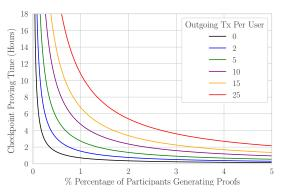
Fig. 6: Estimated time required to create a checkpoint consistency proof with a fraction of users generating proofs in parallel. We assume one user runs one CPU.
