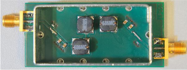
Fig. 2: Third-order (Butterworth Pi) LC low pass filter with cutoff-frequency of  $\sim 100$  Hz.
