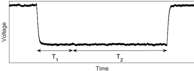
Fig. 3: Exemplary depiction of two measurements, one with and one without low-pass filter, for a measurement interval of 50 ms. Time period  $T_1$  (here 20 ms) corresponds to the interval that is ignored due to the memory effect. Time period  $T_2$  (here 50 ms) corresponds to the measurement interval. All values that are measured in  $T_2$  are averaged to a singular static power value.
