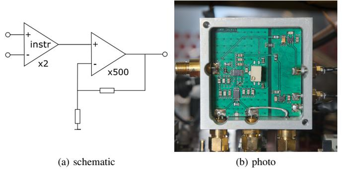
Fig. 1: Low-noise DC amplifier for static power measurements.
