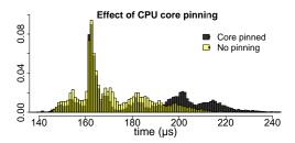
Figure 15: Effect of CPU core pinning on the enclave application. Restricting the enclave application to a specific core has a very minor effect on the observed latency.
