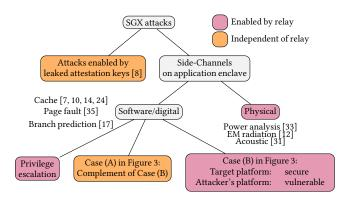
Figure 2: Relay attack implications. The tree shows the types of attacks that are enabled by redirection and ones that are independent of relay.
