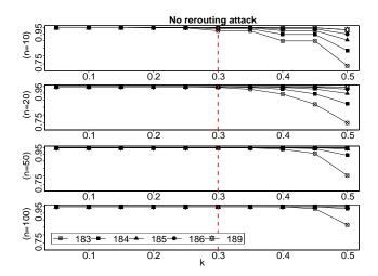
Figure 12: Legitimate attestation success probability for different  $T_{con}$  values. The chosen value  $T_{con} = 186 \ \mu s$  gives success probability 0.99999977 for number of trials at least 15 out of n=50 rounds when k=0.3.
