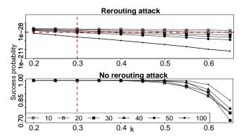
Figure 14: Finding suitable fraction k. The graph shows the legitimate enclave's success probability in an ideal scenario and the attacker's success probability in rerouting attack scenario with varying k.
