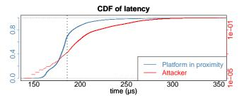
Figure 13: Cumulative distribution function for latencies. We set the threshold  $T_{con}$  at 183  $\mu s$  which has a cumulative probability of 0.693 in the experiment where no rerouting attack takes place with probability of  $1.33 \times 10^{-4}$ .
