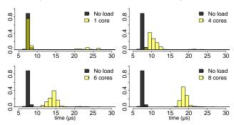
Figure 16: Effect on enclave execution time with different number of stressed CPU cores. Increase system load has a minor effect on observed enclave execution time.
