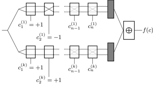
Fig. 1: Schematic representation of an XOR Arbiter PUF with  $k = 2$  parallel arbiter chains.
