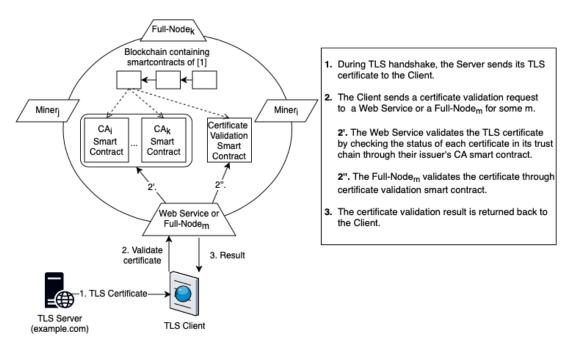
Fig. 1: The TLS System of Yakubov et al.'s Scheme
