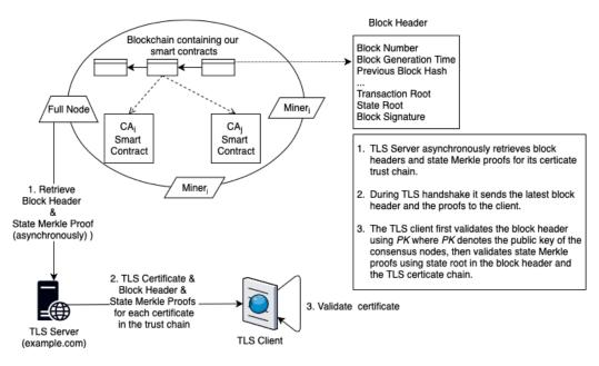
Fig. 2: The TLS System of KORGAN
