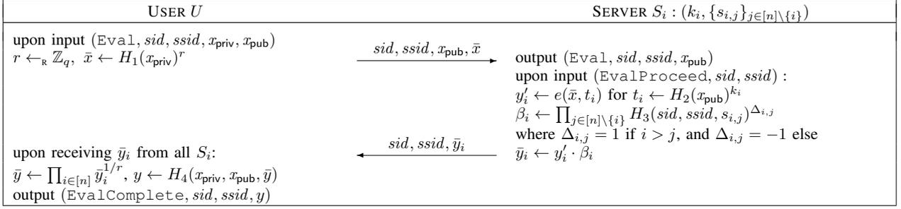
Figure 4: Evaluation protocol of our DH-dpOPRF construction.
