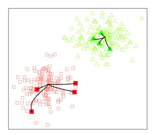
Fig. 1. Illustration of the Mean-shift Algorithm
