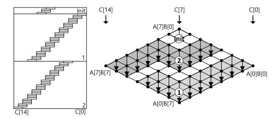
Figure 2: 256-bit Operand Caching multiplication at the word-level where e is 3 on ARM Cortex-M4 [FA17], fait: initial block; (1)  $\rightarrow$  (2): order of rows.
