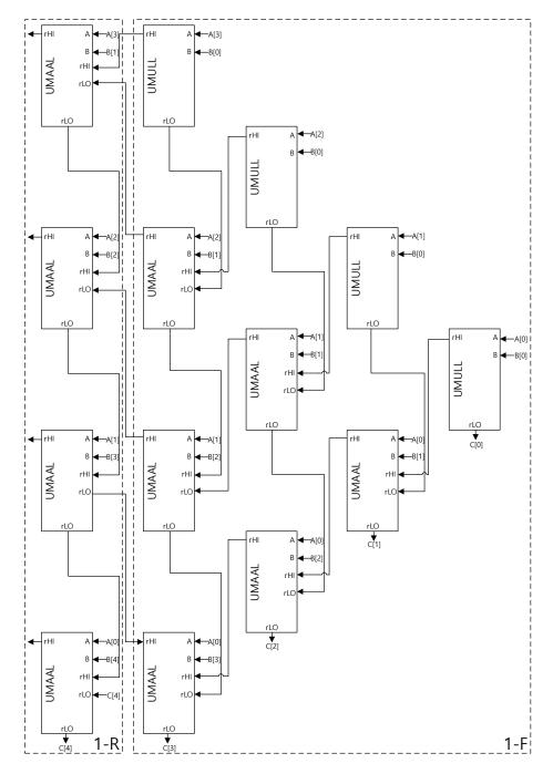
Figure 6: 4-word integers with the product scanning approach using the <code>UMULL</code> and <code>UMAAL</code> instructions for front part of OC method.
