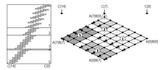
Figure 3: 256-bit Operand Scanning multiplication at the word-level on ARM Cortex-M4 [HL19],  $\textcircled{1} \rightarrow \textcircled{2} \rightarrow \textcircled{3} \rightarrow \textcircled{4} \rightarrow \textcircled{5}$ : order of rows.
