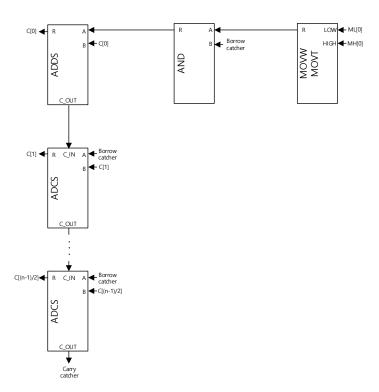
Figure 12: Initial part of of step (2) in 512-bit modular addition/subtraction on ARM Cortex-M4 (i.e.  $C[0\sim(n-1)/2]+(P[0\sim(n-1)/2]\&M))$ .
