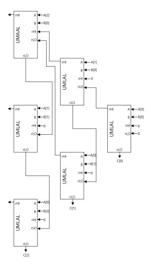
Figure 5: 3-word integers with the product scanning approach using the UMLAL and UMAAL instructions for front part of OC method [FA17].
