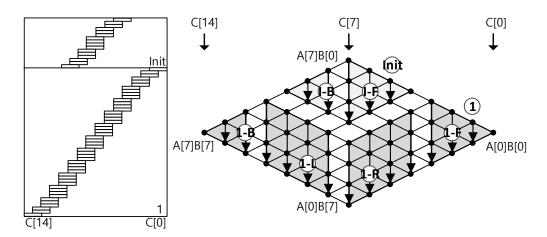
Figure 4: Proposed 256-bit Refined Operand Caching multiplication at the word-level where e is 4 on ARM Cortex-M4, [mit: initial block; []: order of rows; [F]: front part; [R]: middle right part; []: middle left part; []: back part.
