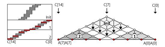
Figure 9: 255-bit proposed squaring at the word-level on ARM Cortex-M4, (nit: initial block; (1)  $\rightarrow$  (2): order of rows.
