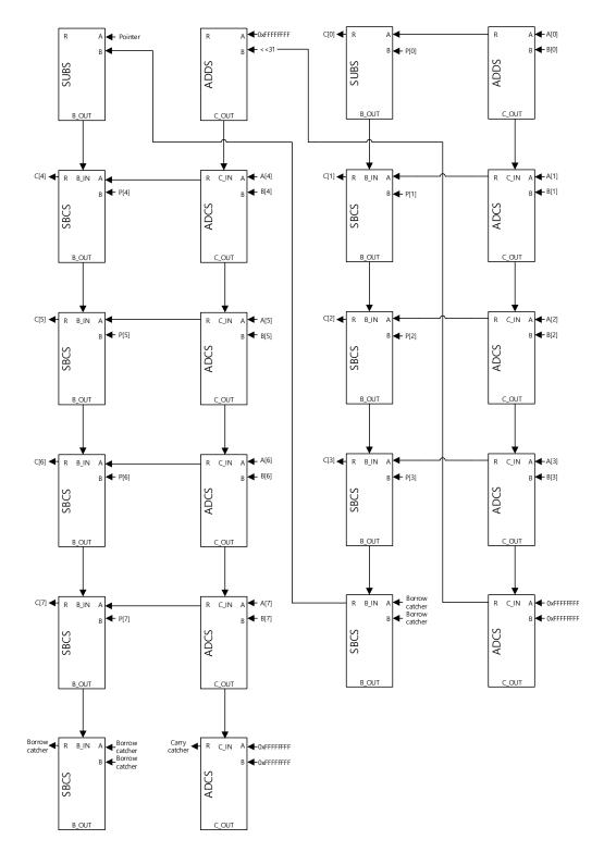
Figure 11: Initial part of step (1) in 512-bit modular addition on ARM Cortex-M4 (i.e.  $A[0{\sim}7]+B[0{\sim}7]-P[0{\sim}7]$ ).
