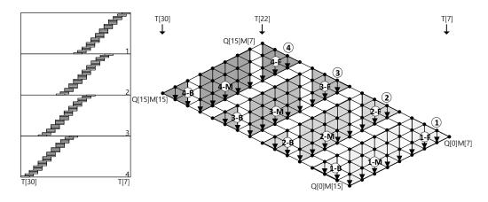
Figure 10: 503-bit "SIDH-friendly" Montgomery reduction at the word-level, where d is 4 on ARM Cortex-M4,  $(1) \rightarrow (2) \rightarrow (3) \rightarrow (4)$ : order of rows; (F): front part; (M): middle part; (B): back part; where M, R, T, and Q are modulus, Montgomery radix, intermediate results, and quotient  $(Q \leftarrow T \cdot M' \mod R)$ .
