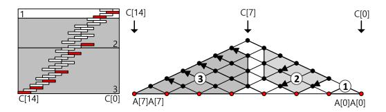
Figure 8: 256-bit Operand Scanning squaring at the word-level on ARM Cortex-M4,  $(1) \rightarrow (2) \rightarrow (3)$ : order of rows [HL19].
