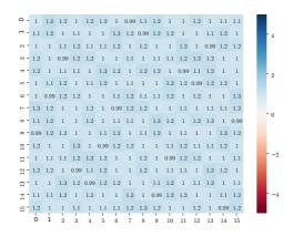
**Figure 2:** Theoretical index-dependent means from the equation system for our four-round distinguisher for the AES, in multiples of  $|\mu_{AES} - \mu_{rand}|$  deviations from the mean of the PRP. Each cell represents the result for the active input cell in the plaintexts (**y**-axis) and the tested inactive cell (**x**-axis) after four rounds without the final MixColumns operation. 1.0 means that the distinguisher matches our prediction closely.
