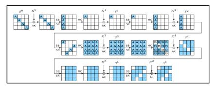
Figure 7: Six-round distinguisher. Darkened cells represent bytes with active (non-zero) difference, white cells represent bytes with zero difference.
