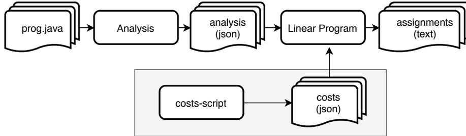
**Figure 4.** Implementation Overview: The analysis takes a Java program as input and outputs a def-use graph (along with related information). The linear program takes as input analysis information and costs, and outputs the optimal assignment.
