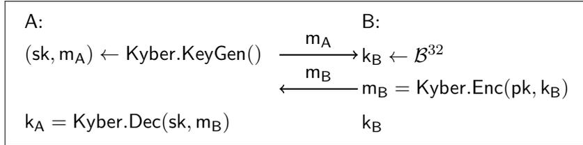
Figure 16: The figure shows a Kyber based key agreement protocol between parties A and B.
