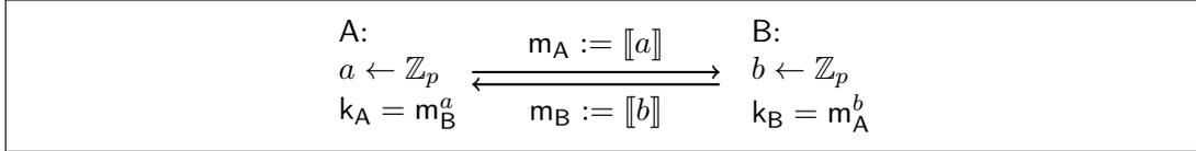
Figure 13: The figure shows the Diffie-Hellman key exchange. Correctness follows from  $k_A = \llbracket ab \rrbracket = k_B$ .
