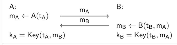
Figure 3: The figure shows a key agreement protocol between parties A and B with random tapes  $t_A$  and  $t_B$ . Correctness requires  $k_A = k_B$ .
