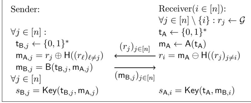
Figure 8: The figure depicts a 1 out of  $n$  OT using a UKA = (A, B, Key) and a random oracle  $\mathbf{H} : \mathcal{G}^{n-1} \rightarrow \mathcal{G}$ , where  $\mathcal{G}$  is a group with operations  $\oplus, \ominus$ . By the correctness of the UKA scheme,  $k_{A,i} = k_{B,i}$  holds. In case of a one round UKA the messages can be sent simultaneously.
