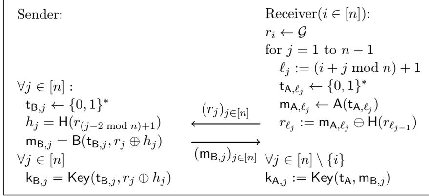
Figure 14: The figure shows a  $n - 1$  out of  $n$  OT using a UKA = (A, B, Key) and a random oracle  $H : \mathcal{G} \rightarrow \mathcal{G}$ , where  $\mathcal{G}$  is a group with operations  $\oplus, \ominus$ . By the correctness of the UKA scheme,  $k_{A,i} = k_{B,i}$  holds. The scheme can be transformed in the same way in a one-round scheme given a one-round UKA as in the 1 out of  $n$  OT case in [Section 4](#).
