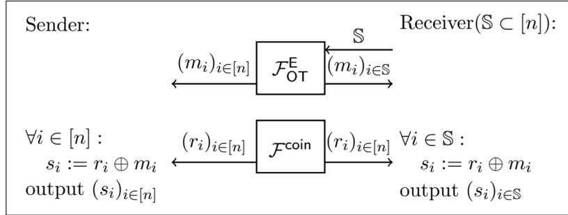
Figure 6: Uniform OT protocol  $\Pi_{k,n}^U$  in the  $\mathcal{F}_{\text{OT}}^E, \mathcal{F}^{\text{coin}}$  hybrid (Definition 2.4). For all  $i \in [n]$ ,  $r_i$ ,  $m_i$  and  $s_i$  are in  $\{0, 1\}^\ell$ .
