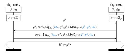
Figure 3: Sketch of STS-ISO [26], which includes the identities of the communicating parties.
