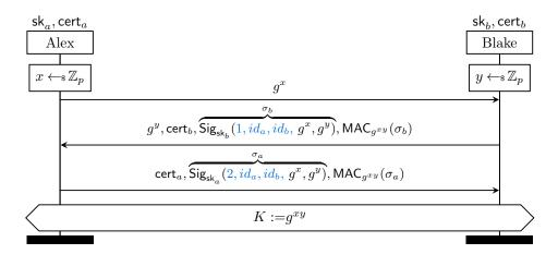
Figure 2: Sketch of STS-ID [26], which includes the identities of the communicating parties in the MAC.
