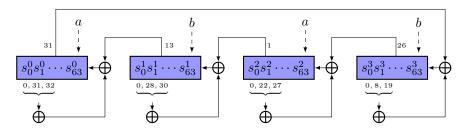
Fig. 5: Schematic of HERN state update function
