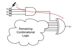
Fig. 3: Fault propagation through S-Box Polynomials. The input pattern causing the propagation is shown in blue. The stuck-at fault type is shown in red.
