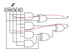
Fig. 4: Fault propagation through masked AND gate.
