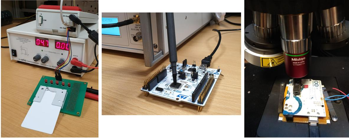
(a) Voltage glitch on a smart card (b) Electromagnetic pulse injection on a microcontroller (c) LASER fault injection on a microcontroller
