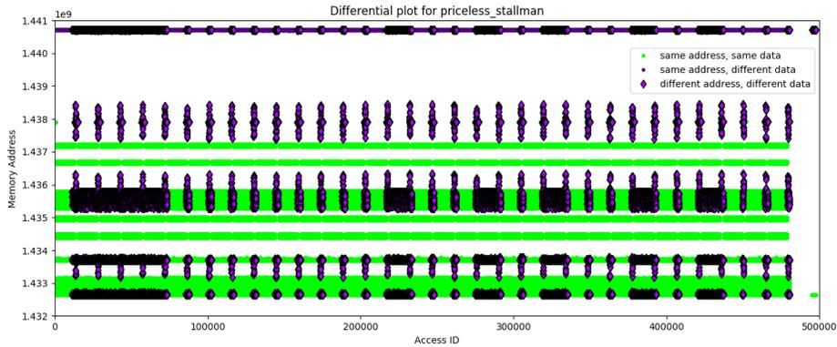
Fig. 5: Difference plot for `priceless_stallman`. Accumulation of dark spots indicates a change of data and control flow whereas green regions resemble constant parts of the implementation. We successfully recovered the key using a second-order analysis of the first quarter of the heavily changing region in the beginning (approx. 20 000 samples).
