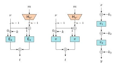
**Fig. 1.1.** (Left): nEHtM MAC based on block cipher  $\mathsf{E}_k$ ; (Middle): nEHtM<sub>p</sub> MAC based on single public random permutation  $\pi$ ; (Right): 2-round iterated even mansour cipher.
