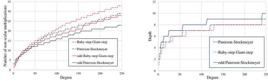
(a) The number of non-scalar multiplications of various evaluation algorithms (b) The depth of various evaluation algorithms
