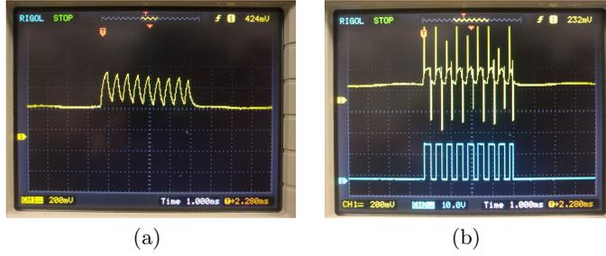
**Fig. 9.** Waveform of the pulse captured by the simple photoreceiver and comparator output. (a) Raw output of the photoreceiver, and (b) raw output (yellow) and comparator output (blue), with the corresponding waveform in Fig. 10.
