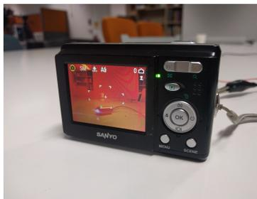
**Fig. 19.** Infrared viewer viewing a light emitting infrared laser module.
