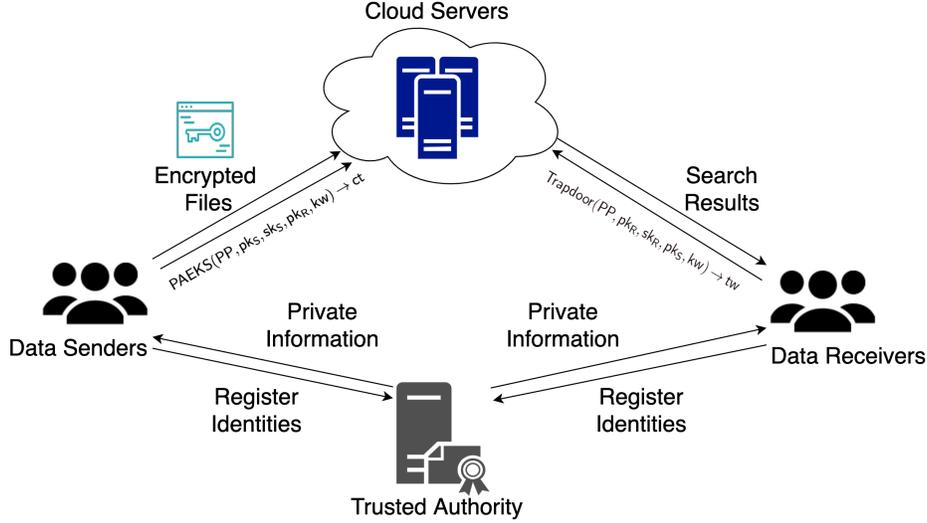
Fig. 2. System model for the proposed PAEKS scheme.
