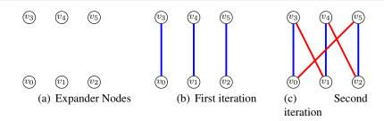
Fig. 3: Illustration of construction of a 2-regular Random Bipartite Expander (Algorithm 1) with six nodes through k = 2 iterations.
