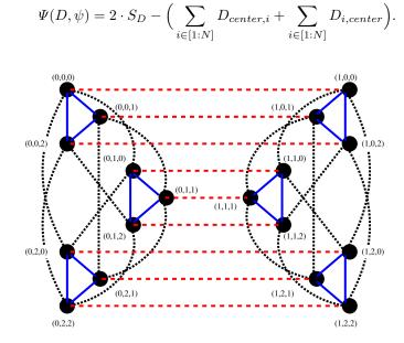
Fig. 4: HyperX topology illustration of L = 3 dimensions with  $S_1 = 2, S_2 = S_3 = 3$ . There are  $N = \prod_{i=1}^{L} S_i = 2 \cdot 3 \cdot 3 = 18$  nodes, each represented by three coordinates. Links along the different dimensions are shown in different colors and line styles. Each nodes is connected to  $d = \sum_{i=1}^{L} (S_i - 1) = (2 - 1) + (3 - 1) = 5$  other nodes.
