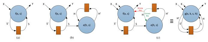
Fig. 1: Logic encryption scheme (a) Original circuit (b) Structural transformation (c) Sequential encryption
