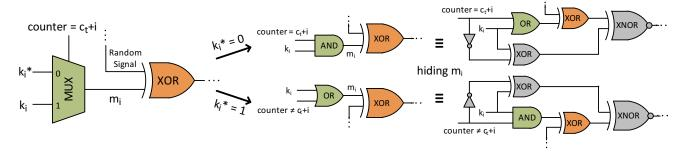
Fig. 2: A structural realization of the proposed practical encryption
