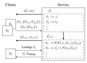
Figure 1: Example showing how Verdict's service updates its state in epoch i for some application-specific policy F. At the end of epoch i, the service broadcasts a new commitment  $C_{i+1}$  and a proof  $\pi_{i+1}$  after incorporating requests from clients  $c_1$  and  $c_2$ . Later, client  $c_3$  can query the server to retrieve the latest value ( $v_2'$ ) associated with label  $\ell_2$ .
