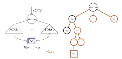
Fig. 11: Position of the forged FORS signature in the SPHINCS<sup>+</sup> tree and of the forged values in the respective FORS tree. Note that the leaves of the tree depend on the forged message, thus the roots that are hashed into the  $pk_{FORS}$  cannot be chosen freely. The first node that can be used for a pre-image attack the sibling  $s_1$  on a second level of a hash tree.
