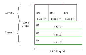
Fig. 9: Magic state distillation scheme for attacking SPHINCS<sup>+</sup>-128.
