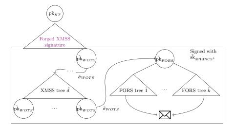
Fig. 6: Forged SPHINCS<sup>+</sup> signature using a forged XMSS signature.
