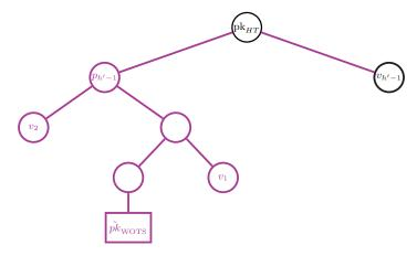
Fig. 7: Structure of a forged XMSS signature.
