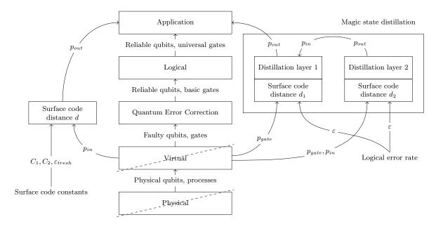
Fig. 3: Layered architecture for quantum computers including parameters for the error correction layer (left) and exemplary magic state distillation (right).
