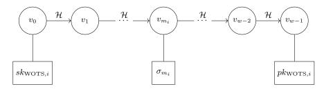
Fig. 8: Structure of one hash chain of a WOTS instance.  $sk_{\text{WOTS},i}, pk_{\text{WOTS},i}, m_i$  and  $\sigma_{m_i}$  are the secret key, public key, message and signature of the *i*-th block of the WOTS scheme with block length  $\log_2 w$ .
