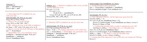
Fig. 6: Our linked attestation scheme for platforms with 2 types of components: VMs (stored in  $S_1$ ) and hypervisors (stored in  $S_2$ ). Each type of component attests via a different **aLAttest** algorithm, the main difference between them being that the hypervisor embeds a list of public keys in its nonce.
