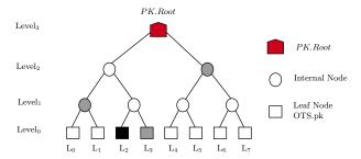
Fig. 2: A one layer XMSS-T, where the leaf nodes are the WOTS-T public keys. The nodes colored in gray are the authentication path for signing with leaf node  $L_2$ .
