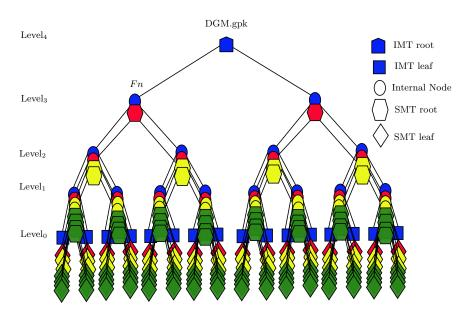
Fig. 5: Simplified DGM example of height 4 with 42 SMTs, 112 signing leaves, and fallback nodes uniformly distributed across the internal IMT nodes
