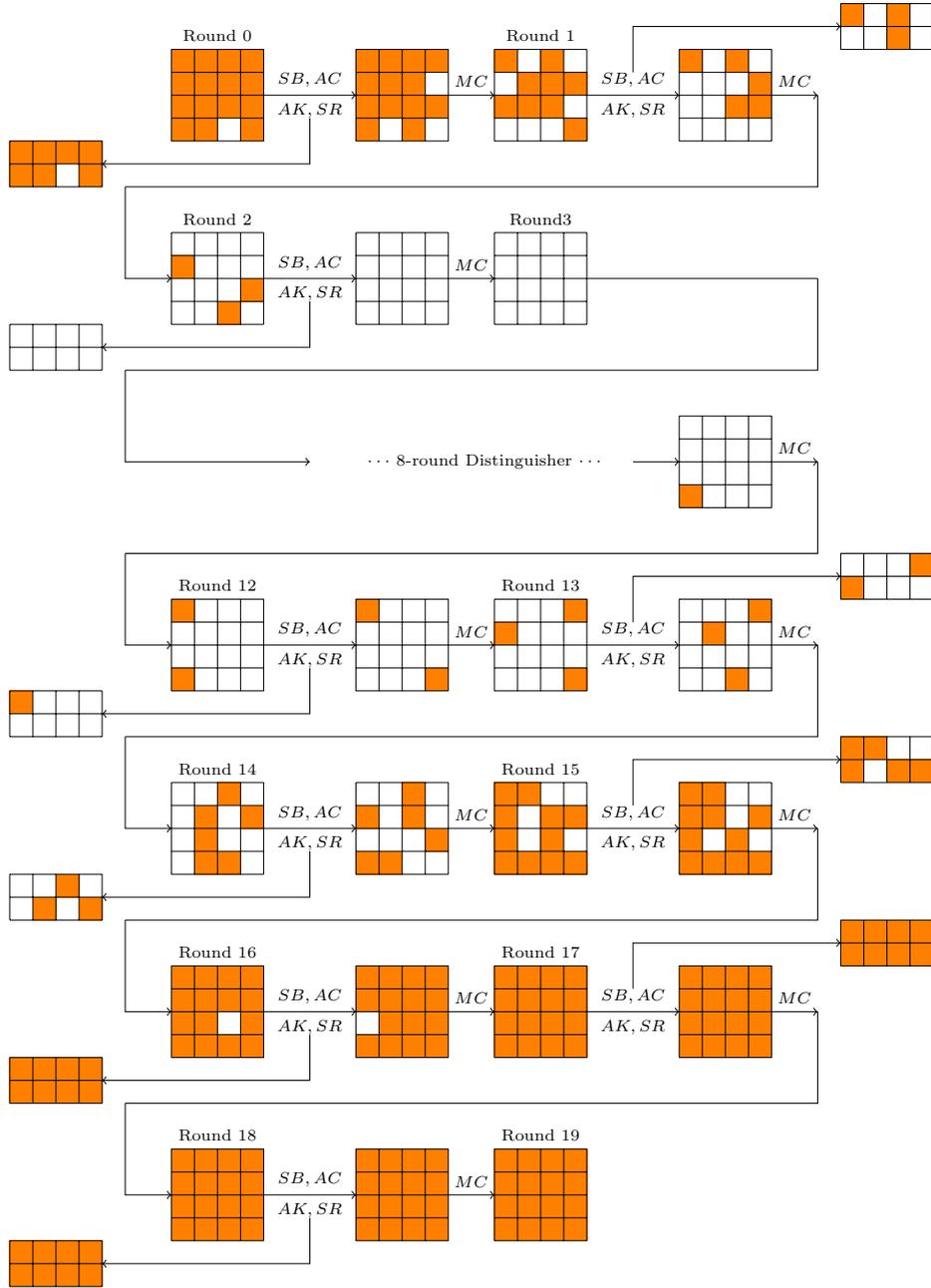
**Fig. 27:** Gussed values for *DS*-MITM attack on 19-round SKINNY-128-256: Derive  $k_{E_0}$  and  $k_{E_2}$  from Figure 26. The sub-keys marked in orange must be guessed (without key-bridging). With the knowledge of these nibbles, we can derive the values of those nibbles of  $P^0$  marked in orange, from which we can determine all red nibbles in Figure 26.
