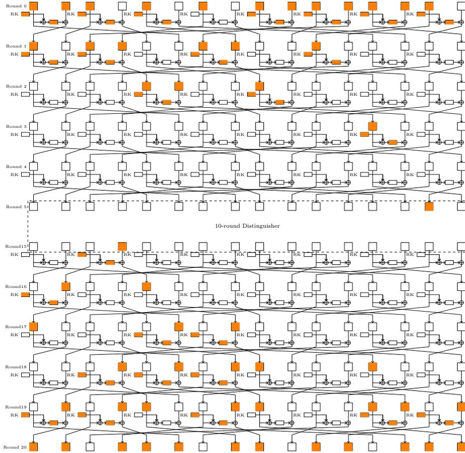
**Fig. 23:** Gussed values in *DS*-MITM attack on 20-round TWINE-80: Derive  $k_{E_0}$  and  $k_{E_2}$  from Figure 22. The sub-keys marked in orange must be guessed (without key-bridging). With the knowledge of these nibbles, we can derive the values of those nibbles of  $P^0$  marked in orange, from which we can determine all blue nibbles in Figure 22.
