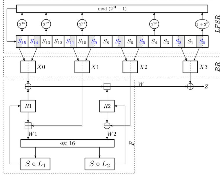
**Fig. 12:** The keystream generation phase of ZUC stream cipher
