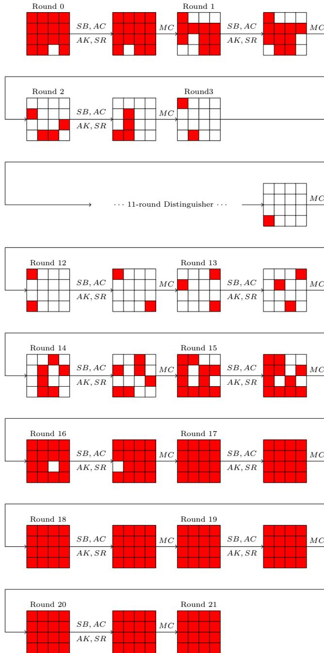
**Fig. 30:** Key recovery for DS-MITM attack on 21-round SKINNY-64-192: Backward differential and forward determination relationship in the outer rounds based on the 8.5-round distinguisher in Figure 29 as  $E_1$  in the middle. Cells in  $\text{Guess}(E_0)$  and  $\text{Guess}(E_2)$  are marked in red.
