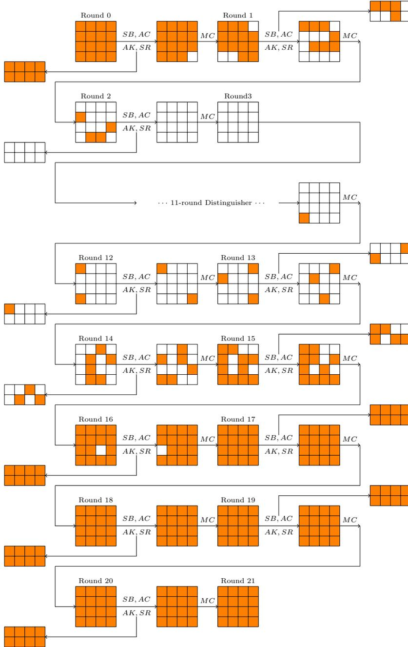
**Fig. 31:** Gussed values for  $DS$ -MITM attack on 21-round SKINNY-64-192: Derive  $k_{E_0}$  and  $k_{E_2}$  from Figure 30. The sub-keys marked in orange must be guessed (without key-bridging). With the knowledge of these nibbles, we can derive the values of those nibbles of  $P^0$  marked in orange, from which we can determine all red nibbles in Figure 30.
