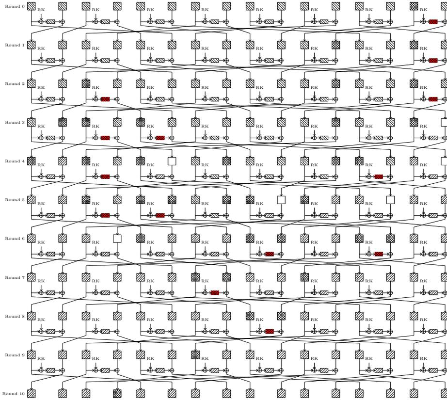
**Fig. 21:** Distinguisher for *DS*-MITM attack on 20-round TWINE-80: A 10-round *DS*-MITM distinguisher for TWINE-80 with  $\mathcal{A} = [14]$  (the nibble denoted by crosshatch in round 0),  $\mathcal{B} = [3]$  (the nibble denoted by crosshatch in round 10), and  $\text{Deg}(\mathcal{A}, \mathcal{B}) = 14$  (the nibbles marked in red).
