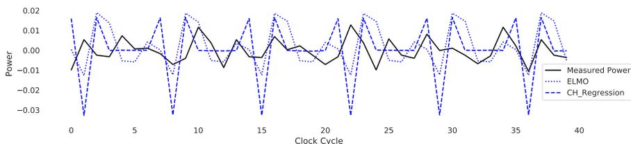
Fig. 9: Power trace for real measured compared to ELMO and  $L_{CH}(X)$
