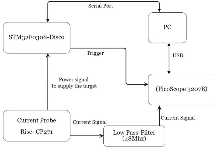
Fig. 2: Setup Block Diagram
