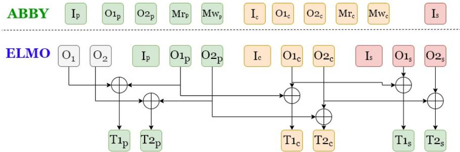
Fig. 4: ABBY vs ELMO features to profile power consumption of the chip
