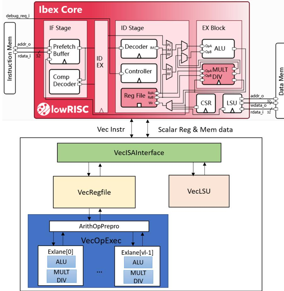
Fig. 1: The architecture of the SIMD RISC-V based Processor.
