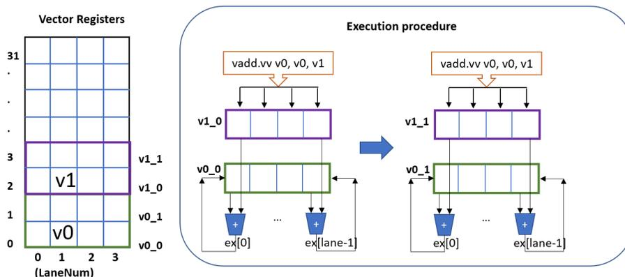
Fig. 2: Vector register file and address allocation.
