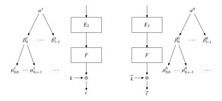
**Fig. 4.** To recover partial key, output mask of  $E_2$ , i.e.,  $\beta^{\iota}$ , is partitioned to *partition* points  $\beta_0^{\iota}, \ldots, \beta_{l-1}^{\iota}, \iota \in \{0, 1\}$ . For every partition points we will find linear trails  $\beta_i^{\iota} \to \mu_{i,j}^{\iota}$  after partition,  $i \in \{0, \ldots, l-1\}$  and  $j \in \{0, \ldots, s-1\}$ .
