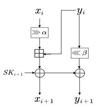
Figure 3: The round function of Speck. For Speck32/64,  $\alpha = 7, \beta = 2$ . For Speck48/X,  $\alpha = 8, \beta = 3$ .
