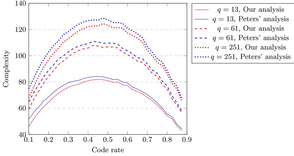
Fig. 3: Complexities to find a minimum-weight codeword, for codes with  $n = 200$ . The minimum distances of the codes have been estimated through the Gilbert-Varshamov bound. The complexity of the algorithms is expressed in bits.
