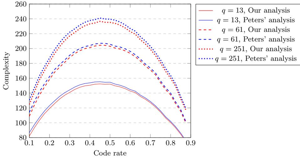
Fig. 4: Complexities to find a minimum-weight codeword, for codes with  $n = 400$ . The minimum distances of the codes have been estimated through the Gilbert-Varshamov bound. The complexity of the algorithms is expressed in bits.
