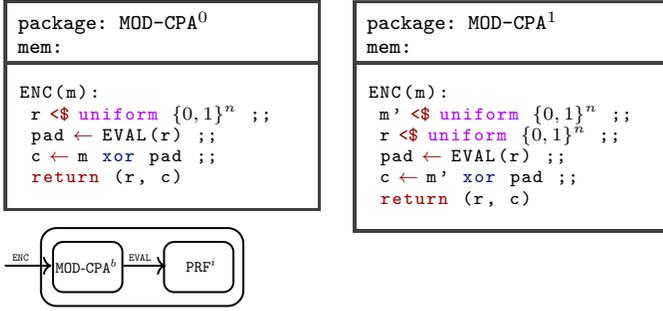
**Figure 7.** Packages MOD-CPA<sup>b</sup> import EVAL from PRF<sup>i</sup>
