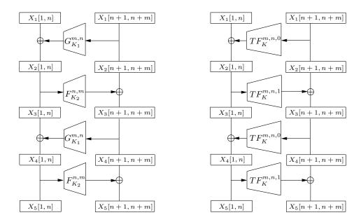
**Fig. 2.** (Left) The 4-round alternating Feistel network  $\mathsf{AFN}^{G^{m,n},F^{n,m},4}$  using a contracting round function  $G^{m,n}$  and an expanding round function  $F^{n,m}$  and two keys  $K_1, K_2$ . (Right) The 4-round alternating Feistel network  $\mathsf{AFN}^{TF^{m,n},4}$  using a tweakable round function  $TF^{m,n}$  and a single key K.
