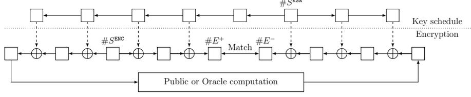
Fig. 1: A high-level overview of the MITM attacks
