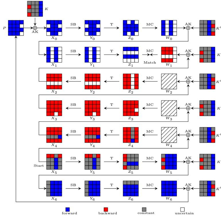
Fig. 17: The 7-round MITM attack on Saturnin-Hash
