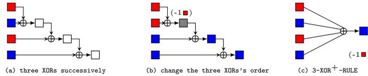
Fig. 5: The inaccuracy of modeling 3-XOR<sup>+</sup> by applying XOR<sup>+</sup> successively
