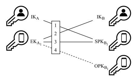
**Figure 3.2:** Extended Triple Diffie-Hellman (X<sub>3</sub>DH) key agreement with user level identity keys and device level ephemeral and prekeys, based on [28].
