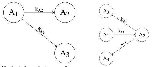
(a) Synchronization via direct messages. Keys may be the same.(b) Synchronization via a device that acts as mirror.
