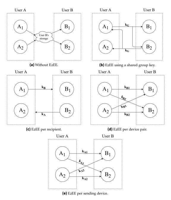
Figure 2.3: Different message sending patterns between two users with two devices each.
