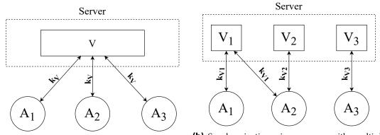
(a) Synchronization via a server with a single vault. (b) Synchronization via a server with multiple vaults.
