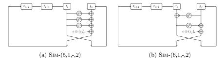
Fig. 4: Novel linear key-expansion algorithms for Sim-(5,1,-,2) and Sim-(6,1,-,2)
