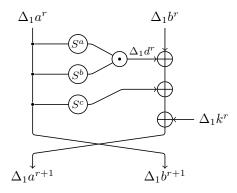
Fig. 1: The round function of a Simon-like cipher and notation for the propagation of RX-differences through it
