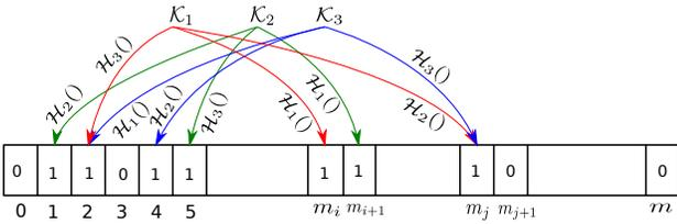
Fig. 3: Bloom Filter: Insertion and Query operations.
