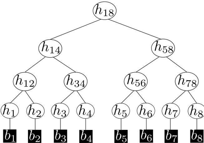
Fig. 1: Construction of the conventional binary Merkle Tree.
