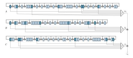
Fig. 2: Overview of the keystream generation of GEA-1 [7].
