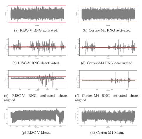
Fig. 7: First-order t-test results of a Keccak-f[800] round. The  $\pm 4.5$  threshold is marked by red lines. Experiments with RNG active use 1M traces, with RNG inactive use 10k traces, and with aligned share evaluations use 100k traces.
