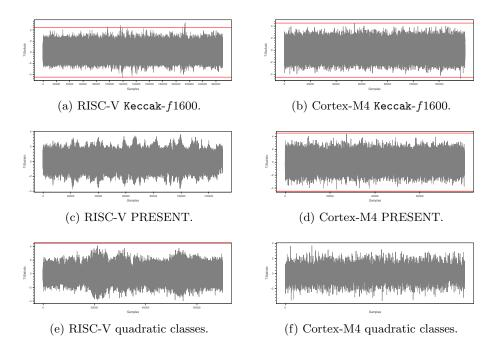
Fig. 8: First-order non-specific, fixed vs. random t-test results on RISC-V and Cortex-M4 cores with 1M traces. The  $\pm 4.5$  threshold is marked by red lines.
