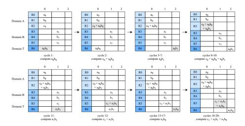
Fig. 5: Outputs  $c_0$  and  $c_1$  of the Toffoli gate. In this masking, registers R0-R2 belong to domain A, R3-R5 belong to domain B, and R6 is a temporary register in domain T.
