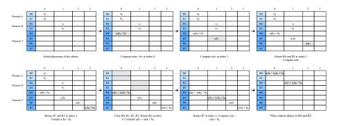
Fig. 4: Methodology for d+1 shares. In this masking, registers R0-R1, R2-R3 belong to domain A and B respectively and R4-R7 are temporary registers in domain T.
