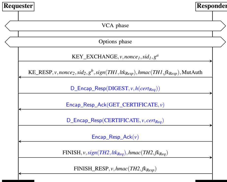
Figure 2: Key Exchange with Mutual Authentication in the optimized encapsulation flow. In the *FINISH* message, if Mutual Authentication is requested (*MutAuth*), the Responder can request digests and certificates for the Requester's public key using encapsulated messages. Additionally, the Requester does sign the transcript *TH2* (which is marked in blue. ) If the Responder already has the certificate of the Requester from another protocol run, they can skip directly to *FINISH*.
