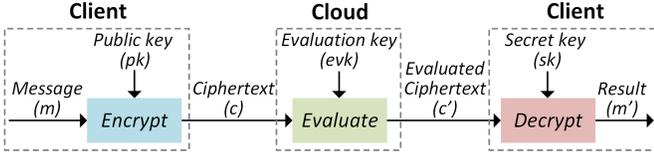
Fig. 1. Homomorphic encryption functions at the client and the cloud. The public key ( $pk$ ) encrypts the message ( $m$ ) to generate the ciphertext ( $c$ ) and the secret key ( $sk$ ) decrypts the received *homomorphically evaluated* ciphertext ( $c'$ ) – both operations execute on the client’s device while *homomorphic evaluations* execute in the cloud.
