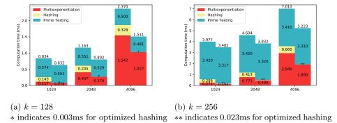
Fig. 5: Comparison of computation time dedicated to each component between non-optimized and optimized implementations for bit-level security k equal to 128 bits in (a) and 256 bits in (b)
