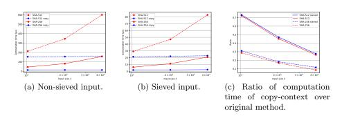
Fig. 4: Comparison of computation time dedicated to hash in the verification algorithm in function of the input size  $\lambda$ .
