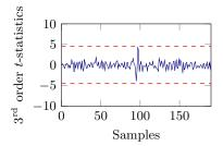
Fig. 15. 2<sup>nd</sup> order TVLA results for the Fig. 16. 3<sup>rd</sup> order TVLA results for the 2<sup>nd</sup> order masked AES S-box based on one 2<sup>nd</sup> order masked AES S-box based on one million simulated traces.
