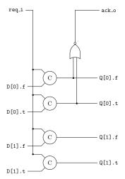
**Fig. 2.** A 2-bit wide strongly indicating asynchronous latch.
