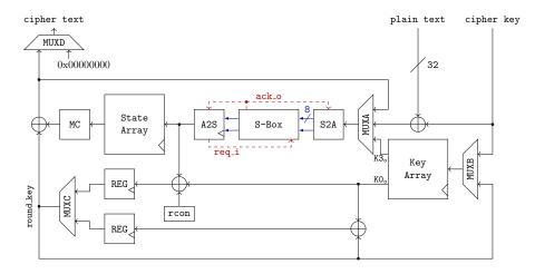
Fig. 11. The LAGS AES128 architecture with a 32-bit data path.
