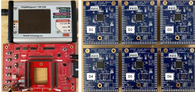
**Fig. 5.** The equipment used in the experiments. The devices  $D_1 - D_5$  are used for the profiling and  $D_6$  is used for the attack.
