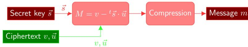
Fig. 5. Overview of the sensitive operations within PKE Decrypt
