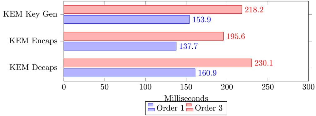
Fig. 2. Performances in milliseconds of our masked ML-KEM-512 at different masking orders
