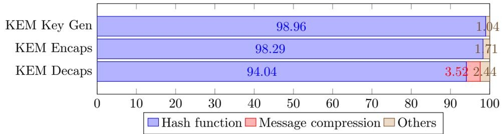
Fig. 3. Impact of Keccak and message compression in percent of time in third order masking
