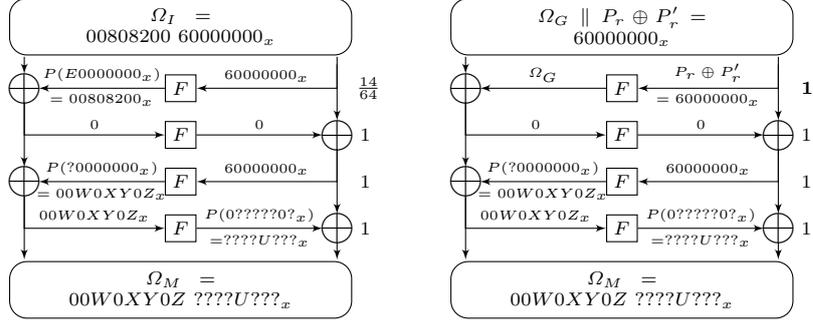
(a) The Differential Characteristic Used in [8]. (b) Our Improved Differential Characteristic.
