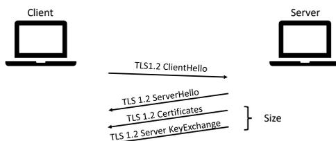
**Fig. 5.** Amplification in TLS 1.2 where the server returns a potentially large post-quantum certificate chain and ephemeral public key while the client has only sent a small ClientHello. The client address is still validated by the TCP handshake.
