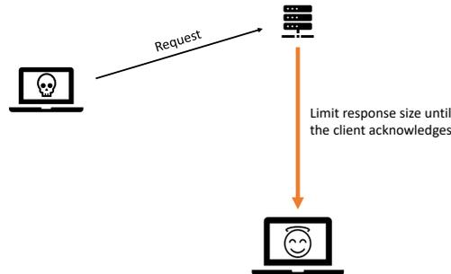
**Fig. 2.** Amplification Protection where the reflector limits the size of the response from a not-yet-validated source and waits for an **Acknowledgement** to limit the impact of a potential reflection amplification attack.
